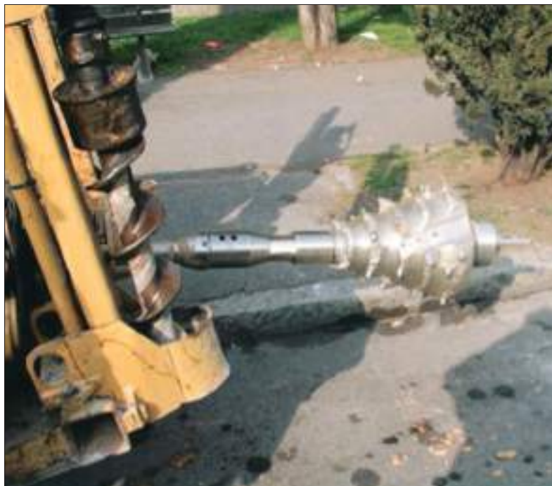
Fig. 7: Alesatore (Fonte 1)
